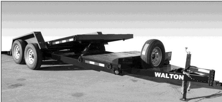
Pivoting Deck Trailer (Tilt-Bed)
