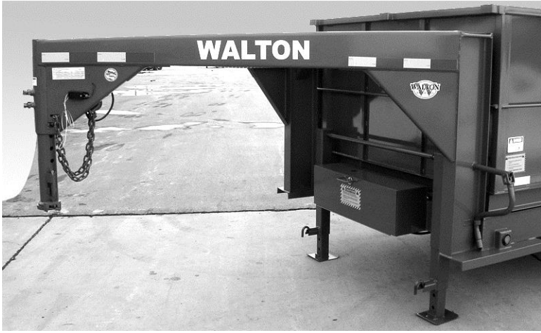
Trailer with Gooseneck Coupler
